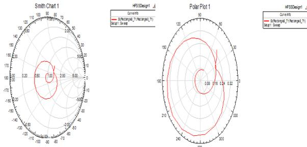
Fig. 11. Smith chart and Polar plots of the dual band MLA in HFSS software
