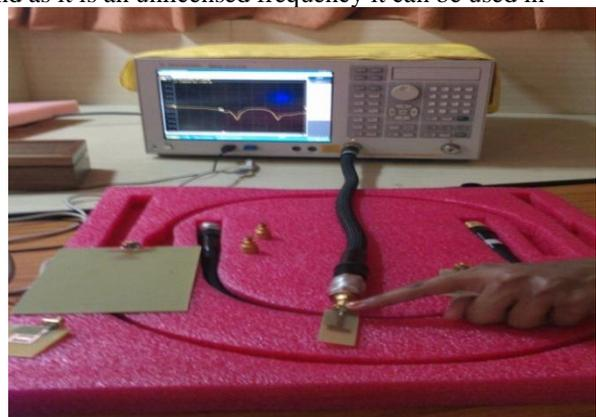
Fig.15. The dual band antenna connected with Vector network analyzer for investigating the results
