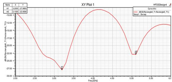
Fig.10. Return loss ( $s_{11}$ ) curve of dual band MLA designed on HFSS software
