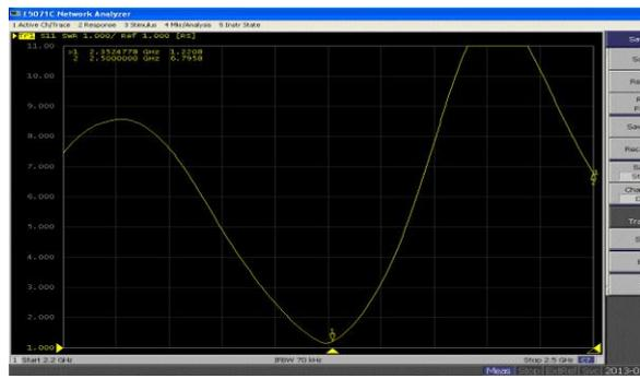
Fig.5. the VSWR plot obtained on the Vector Network Analyzer for the WLAN antenna.
