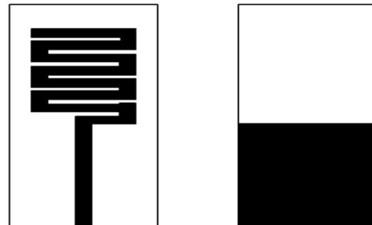
Fig.1. Illustration of a printed meander-line antenna for the WLAN applications (a) Front plane and (b) ground plane.
