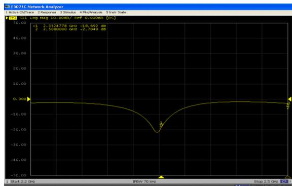
Fig.6. the Return loss plot obtained on the Vector Network Analyzer for the WLAN antenna.
