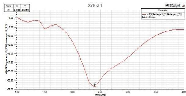
Fig.3. Return loss ( $s_{11}$ ) curve of WLAN antenna designed on HFSS software
