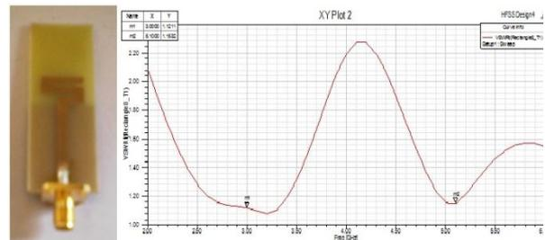
Fig.9. Photograph of a realized dual band meander line antenna on a FR-4 substrate and measured antenna input VSWR on HFSS software.
