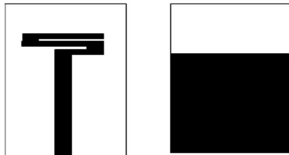
Fig.8. Illustration of a dual band meander-line antenna for wireless applications (a) Front plane and (b) ground plane.
