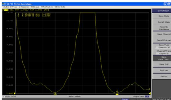
Fig.12. The VSWR plot obtained on the Vector Network Analyzer for the dual band antenna
