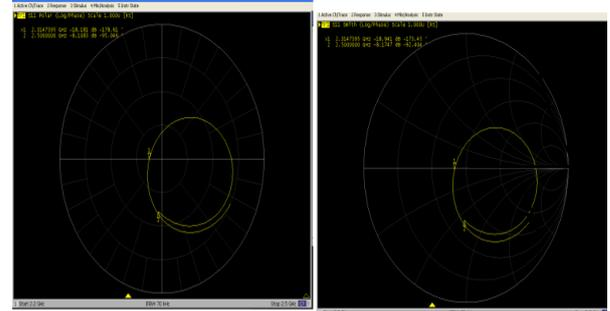
Fig. 7.Smith chart and Polar plots of the WLAN antenna in Network Analyzer.
