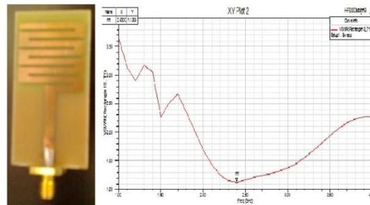
Fig.2. Photograph of a realized WLAN meander line antenna on a FR-4 substrate and measured antenna input VSWR on HFSS software.
