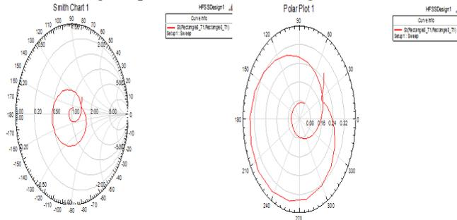
Fig.4.Smith chart and Polar plots of the WLAN antenna in HFSS software
