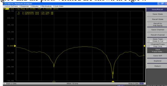
Fig.13. the Return loss plot obtained on the Vector Network Analyzer for the dual band antenna
