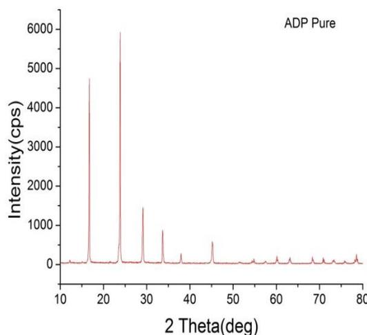
Fig.6. XRD pattern of Pure ADP with ultrasonic irradiation
