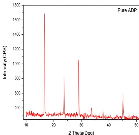
Fig.7. XRD pattern of Pure ADP without ultrasonic irradiation
