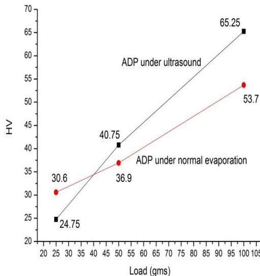
Fig.5. Micro hardness graph
