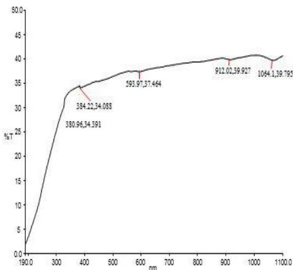
Fig.4. UV spectrum of Pure ADP without Ultrasound
