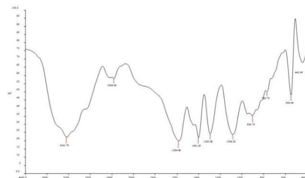
Fig.2. FTIR spectrum of Pure ADP without ultrasonic irradiation
