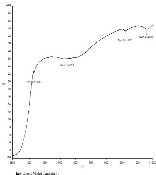
Fig.3. UV spectrum of Pure ADP with Ultrasound
