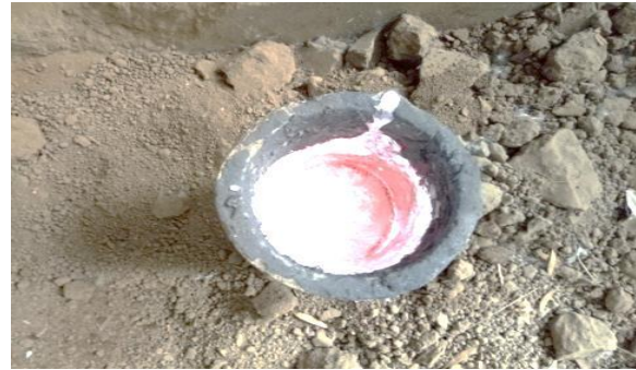
Figure 7 After melting mixture Al 6063+SiC mould
