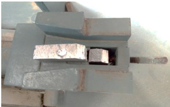
Figure 5 After breaking material on impact (Izod) Test
