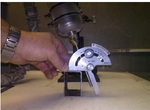
Fig. 3. Nozzle angle setting by means of accessory
