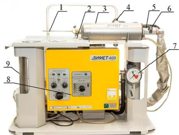
Fig. 2. General view of test facility DYMET–405: 1– nozzle SK-6; 2 – silicone adaptor; 3 – sprayer DM-43; 4- powder delivery button; 5 – powder delivery tube; 6 – sprayer pneumatic valve; 7 – gauge; 8 – monitor and control unit MCU-03; 9 – feeder FV-43.
