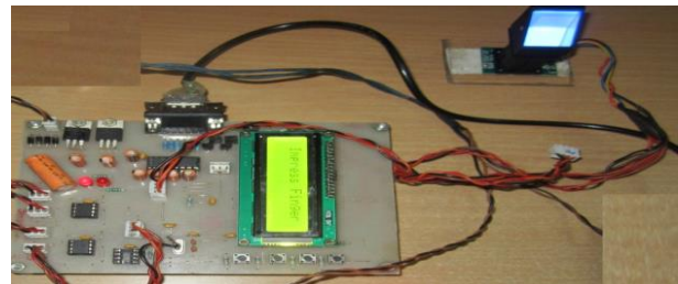
Figure 11: Interfacing of fingerprint module with LPC 2148
