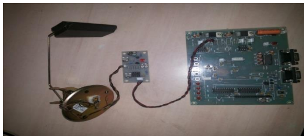
Figure7: Float level Sensor with ARM
