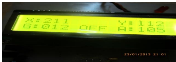
Figure 10: Reading of the acceleration and alcohol sensor
