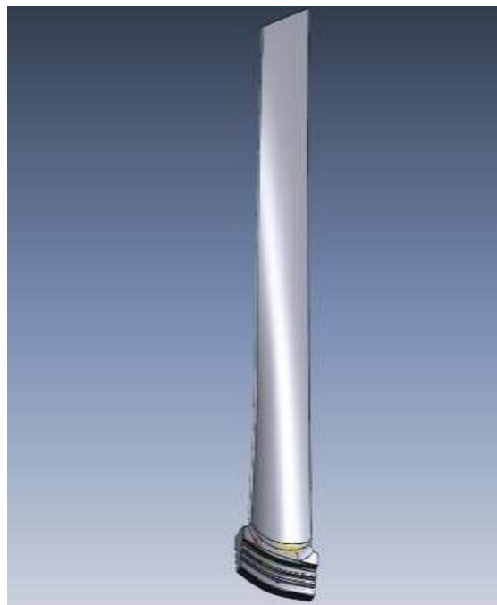
Figure 6: Solid model of the rotor blade
