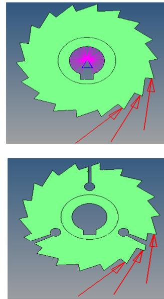
Figure 3: 1.2kN load applied on the saws
