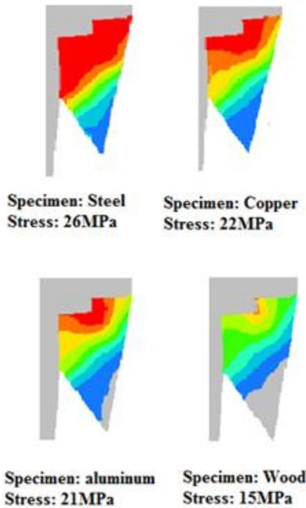
Figure 6: Comparison of stresses in the saw after cutting four different specimens.
