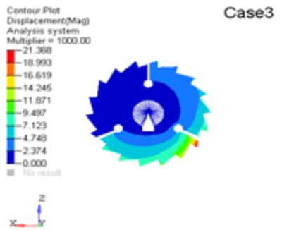
Figure 3.1: Deflection in the saws after the application of 1.2kN load.
