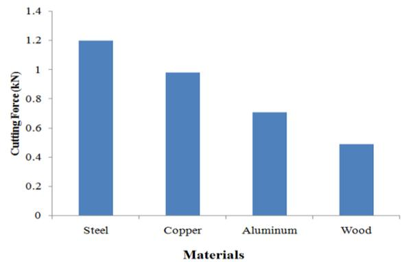
Figure 5: Comparison of cutting force generated while cutting the four different specimens.
