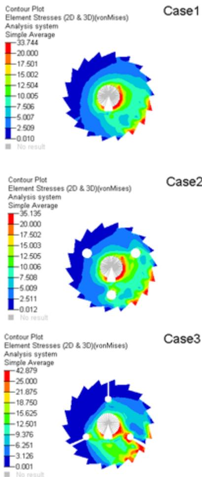
Figure 3.2: Stresses in the saws after the application of 1.2kN load.
