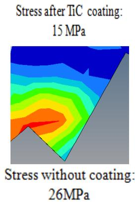
Figure 8: Comparison of stresses with and without coating.
