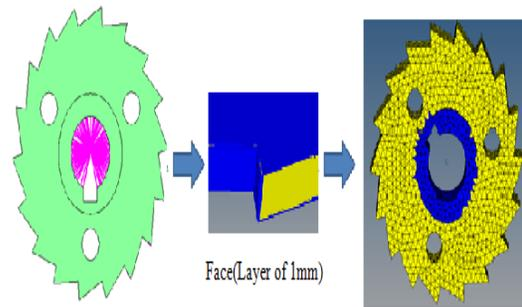
Figure 7: Coating on the circular saw blade with 1mm thickness.
