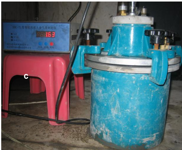
Fig. 2 (a) Test set up for compressive strength of concrete cube specimens (b) Three-point loading flexural testing device and set-up (c) Air content test by pressure method
