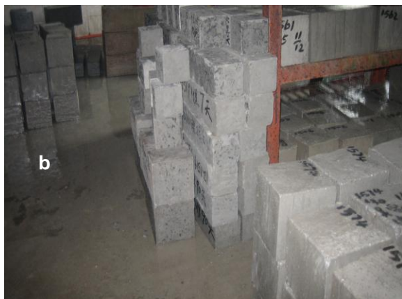
Fig. 1 (a) some concrete samples on the vibrating table (b) some concrete samples in the fog (moist) room.
