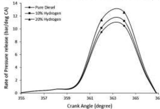
Fig. 10. Rate of pressure release at different hydrogen substitutions
