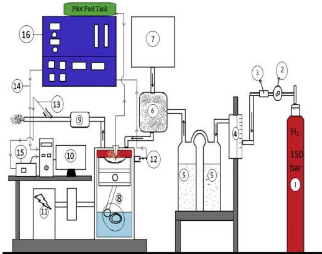
1.H<sub>2</sub> gas cylinder 2.Pressure gauge 3.Back flash arrestor 4.Flow meter 5.Flame arrestor 6.Mixing chamber 7.Air tank 8.Engine 9.Exhaust gas calorimeter 10.PC 11. Eddy current dynamometer 12.Piezoelectric sensor 13.Exhaust gas sensor 14. Sensor to PC 15.Exhaust analyser 16.Control panel
