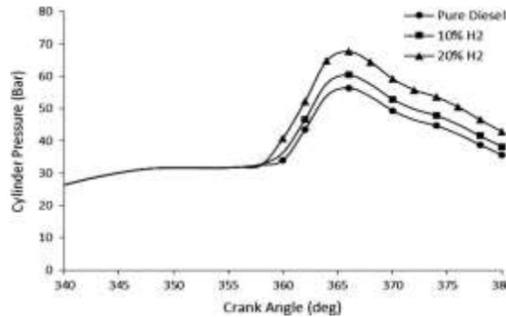
Fig.8. Cylinder pressure vs. crank angle.
