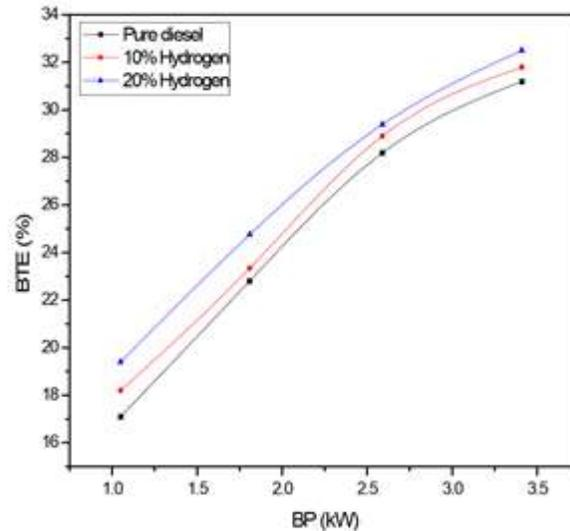
Fig. 3. Variation of brake thermal efficiency with Brake Power
