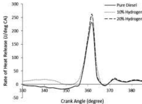
Fig. 9. Rate of heat release at different hydrogen substitutions.
