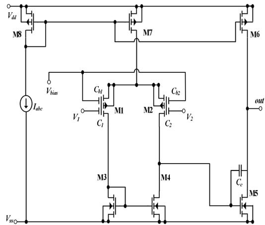
The circuit of two-stage OTA using FG-MOSFETs
