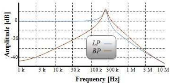
**Figure 5. Simulated frequency responses of low-pass and bandpass signals shown in Figure 4.**
