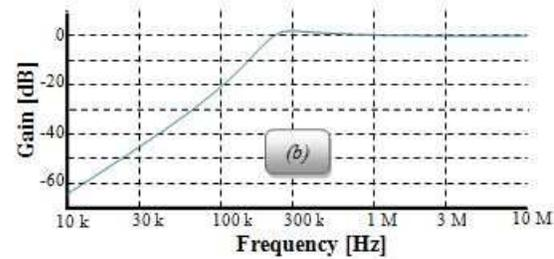
Figure 10. Simulated (a) phase and (b) frequency responses of the HP filter.
