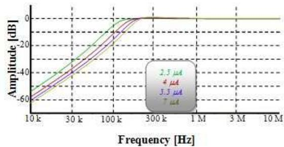
High-pass filter cutoff frequency vs.  $I_{abc1}$  ( $G_{m1}$  is variable).
