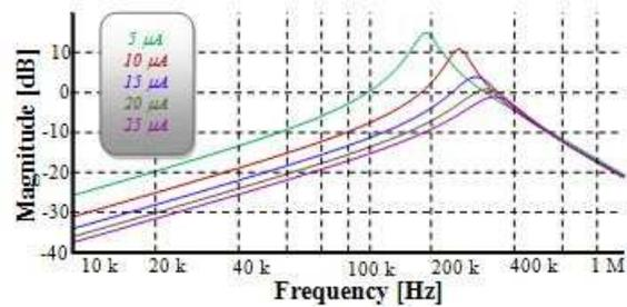
**Figure 7. Bandpass filter when  $I_{abc2}$  is varied ( $G_{m2}$  is variable).**
