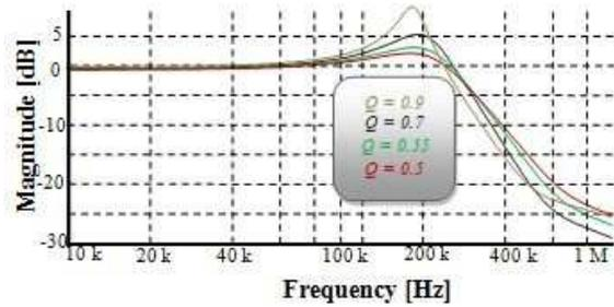
**Figure 6. Low-pass filter peaking vs.  $Q$  ( $G_{m1}$  is variable).**
