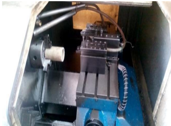
Figure 2 Machining setup of GFRP
