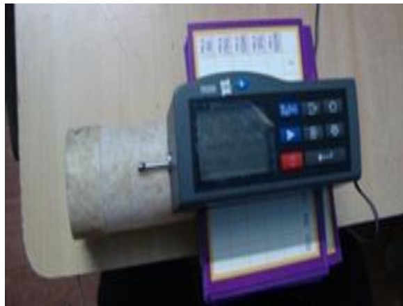
Figure 3 Surface roughness tester setup of GFRP
