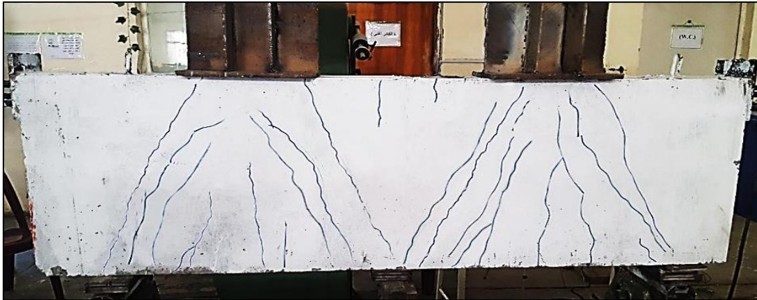
Figure 8 DBU specimen after test
