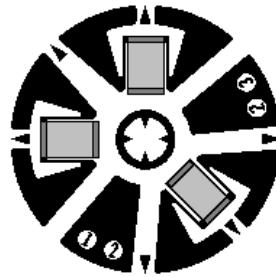
Fig: Strain Gage Arrangement for Measuring Residual Stress
