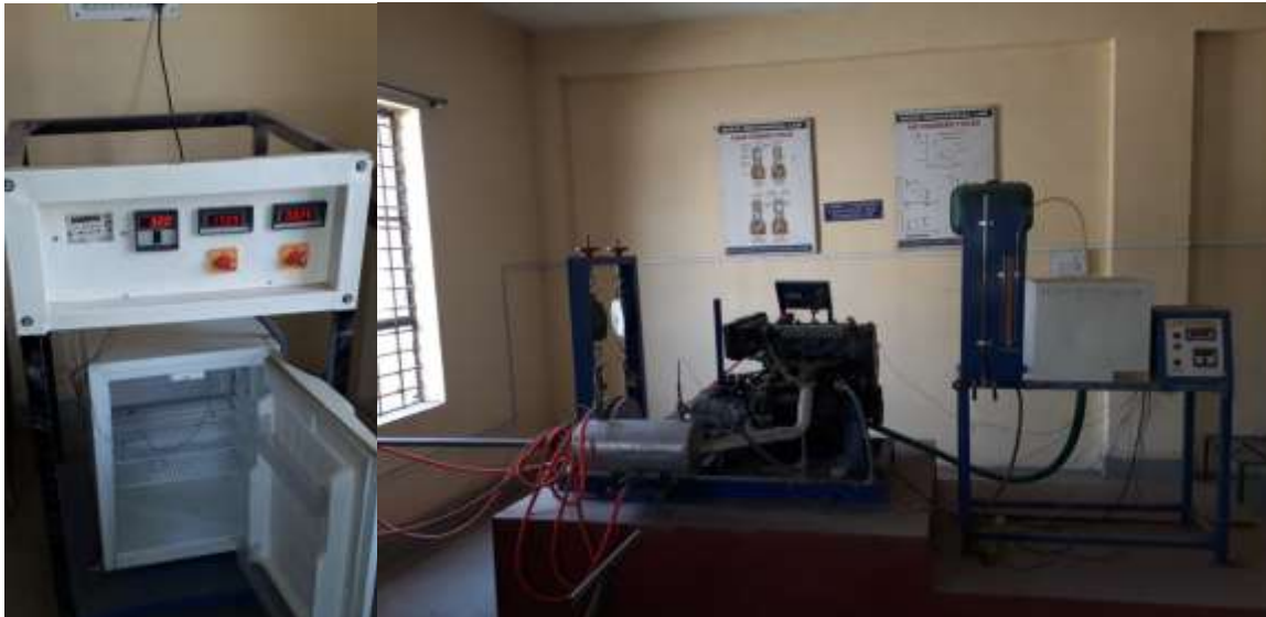
FIG 2 -ACTUAL EXPRIMENTAL SETUP OF 4 STROKE 4 CYLINDER DIESEL ENGINECOUPLED WITH ROPE BRAKE DYNMOMETER AND CONNECTED WITH THREE FLUID VAPOUR ABSORPTION RFRIGERATION SYSTEM
