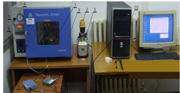
Fig.1. Experimental far-infrared vacuum setup 1-vacuum pump, 2-separator, 3-vacuum chamber, 4-vacuum meter, 5-temperature controller, 6-vacuum regulator, 7-samples, 8-micro-thermocouples, 9-load cell, 10-shelf, 11-heaters, 12-data acquisition system,13-24 bit A/D converter, 14-personal computer
