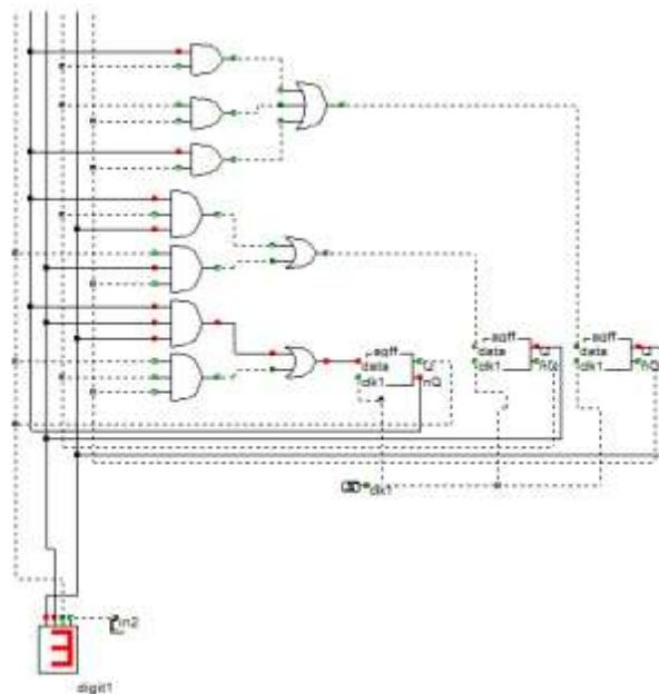
Fig.7. Self-Starting and Self-Correcting Counter with Auto Gated Flip-Flops.
