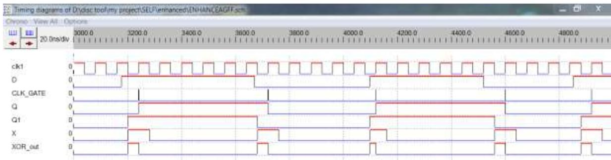
Fig.14.output waveform for enhanced AGFF with the XOR output
