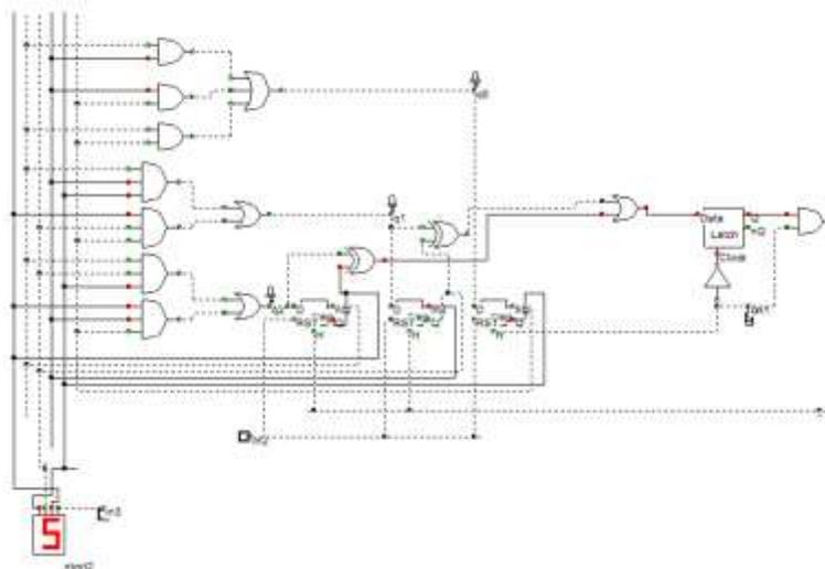
Fig. 4. Self-starting and Self-correcting counter implementation with Data-driven clock gating technique.
