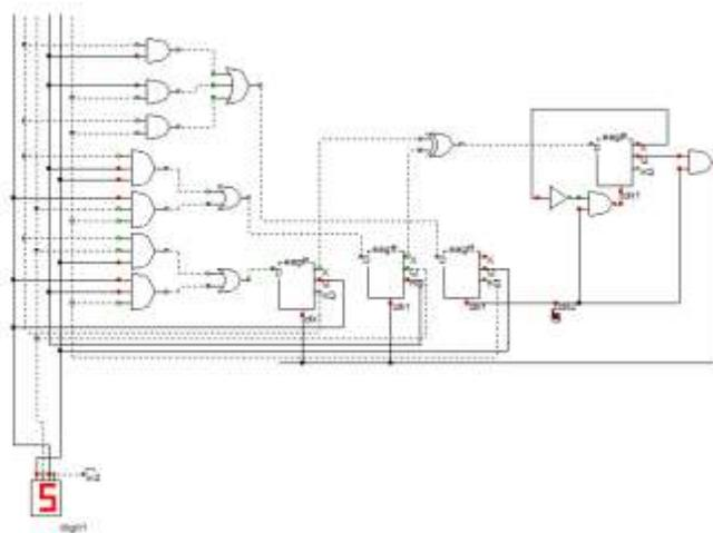
**Fig.10. Self-Starting and Self-Correcting Counter with Look-Ahead clock gating (LACG).**
