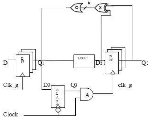
Fig. 3. Circuit implementation of data-driven clock gating.
