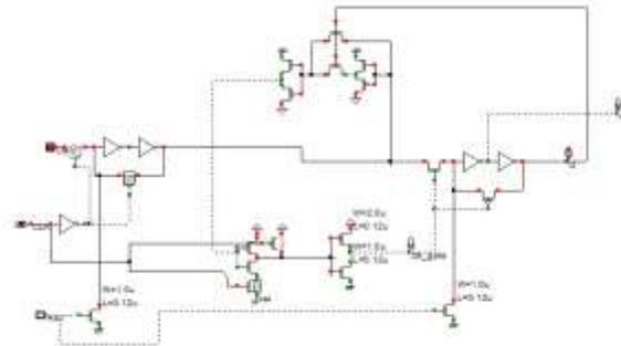
Fig.5. Schematic diagram of Auto Gated Flip-Flop.
