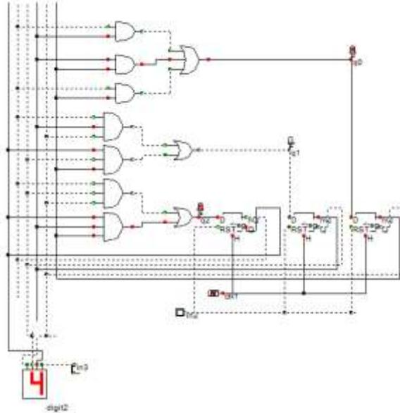
**Fig: 2. Self-starting and Self-correcting counter**
