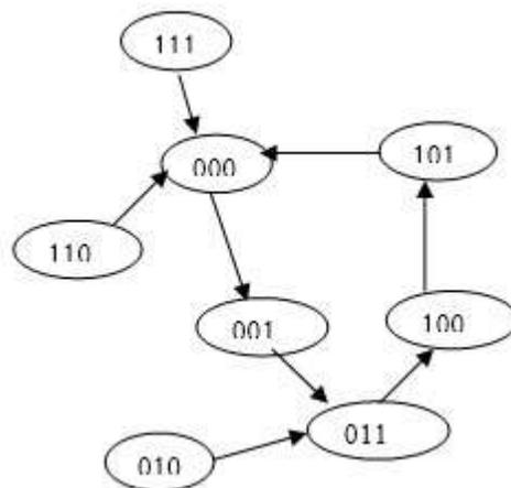
*Fig: 1. State transition diagram of a Self-starting and Self-correcting counter.*
