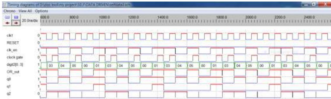
Fig: 12. Simulation result for 3-bit Self-Starting and Self-Correcting Counter with data-driven clock gating.
