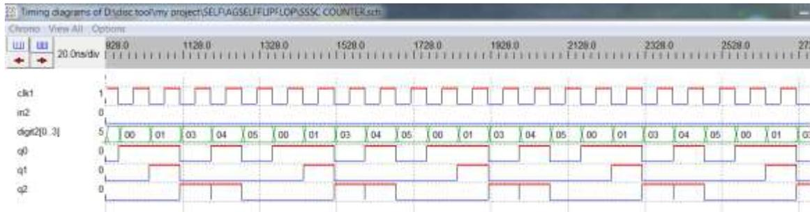
Fig.11. Output waveform for Self-Starting and Self-Correcting Counter circuit
