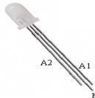
Figure 1: Bicolor LED (Model: SSL-LX5097IGW)
