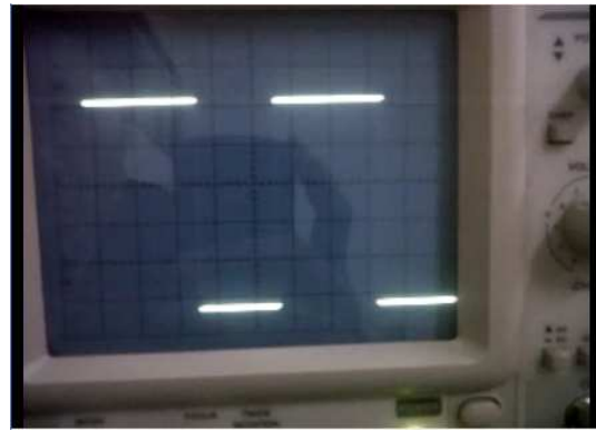
Figure 7. Output with V/Div = 2 V/Div and Time/Div 50 ms/Div
