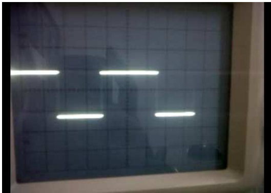
Figure 6. Output with V/Div = 5 V/Div and Time/Div 20ms/Div
