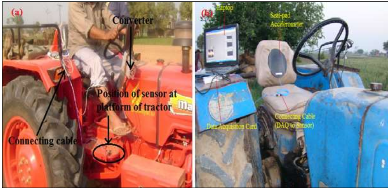
Figure 2. Mahindra Bhoomiputra 265 DI Model tractor on farm field conditions (a) Breaking system arrangement, (b) Seat pad arrangement.
