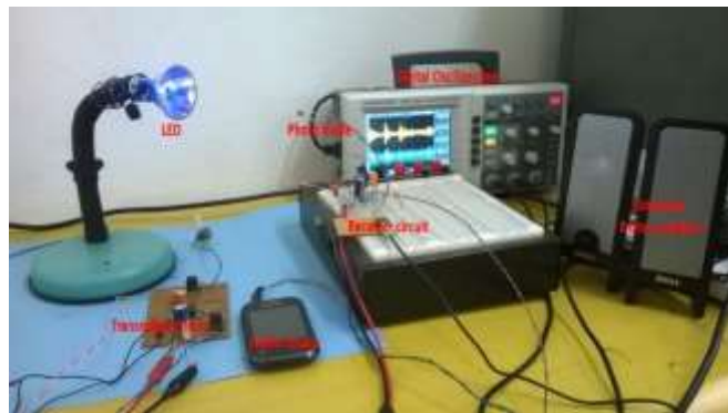
Figure 5. Experimental setup for OLC based stereo audio system.
