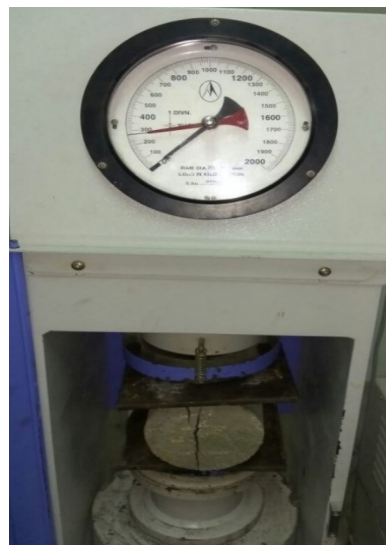
Figure 4 Tensile strength test Setup
