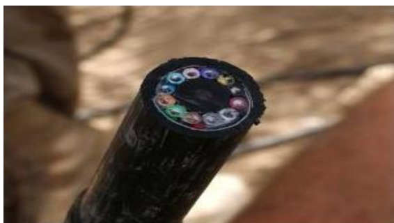
Figure 1. Image of a section of 144 strand optical fibers cable. Each strand is made of optically pure glass and is thinner than a human hair.
