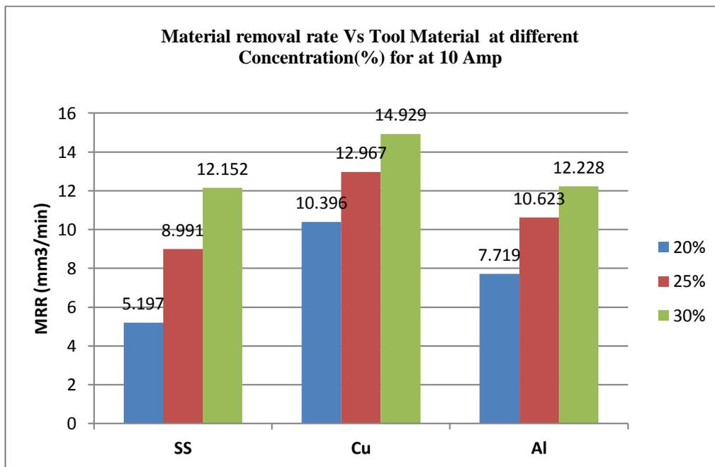
**Fig. 2. Plot between Material removal rate Vs Tool Material at different Concentration (%) for at 10 Amp**
