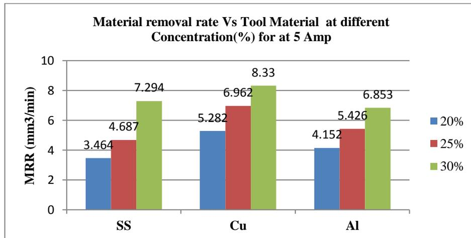
**Fig. 1. Plot between Material removal rate Vs Tool Material at different Concentration (%) for at 5 Amp**
