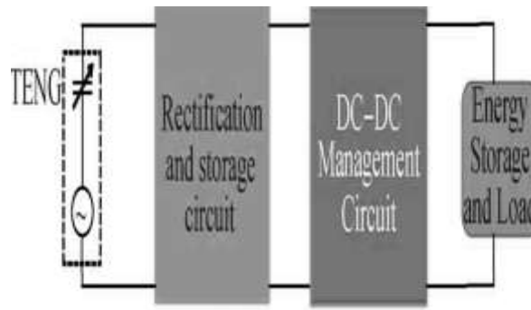
Fig. 7: - Structure of the TENG utilized with power management circuits
