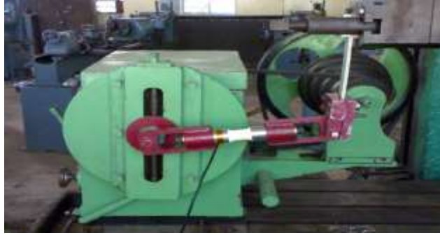
3.6 (a). Eccentric mechanism of the referred test rig design
