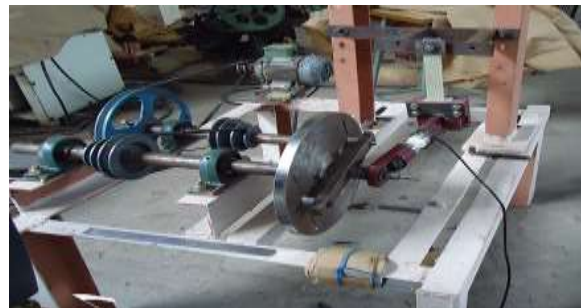
Fig.3.6 Eccentric mechanism and the total Test Rig assembly made in this project work
