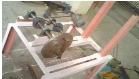
Fig.3.5 power transmission system mounted on base frame
