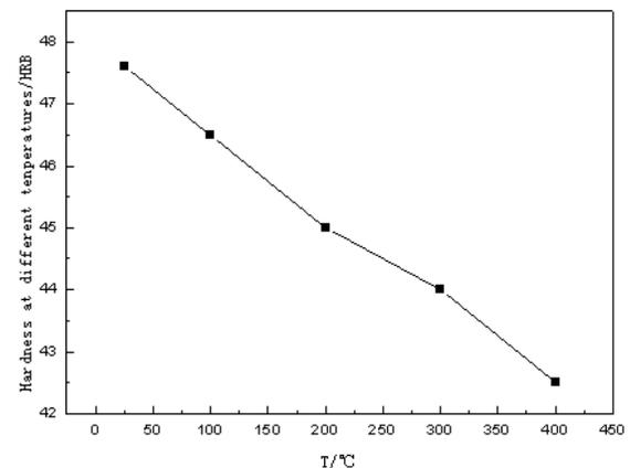
**Fig. 2.2** micro hardness curve of alloy at various annealed temperatures without electric pulse
