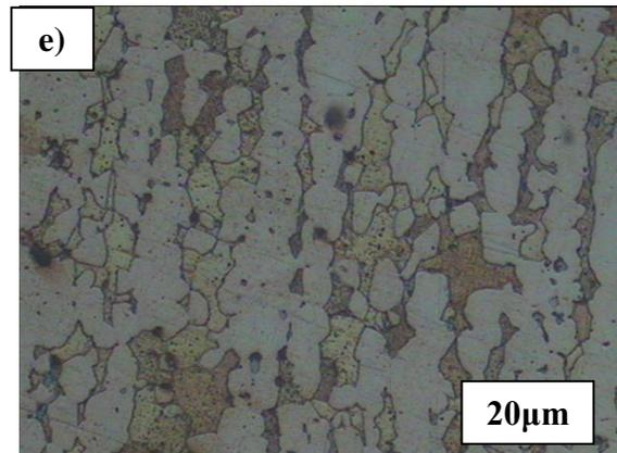
**Fig 2.1** the microstructure of alloy at various annealed temperatures without pulsed and soaked for 30mins
