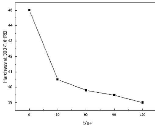
**Fig 5.2** micro hardness curve of alloy at various pulsed time for 300°C
