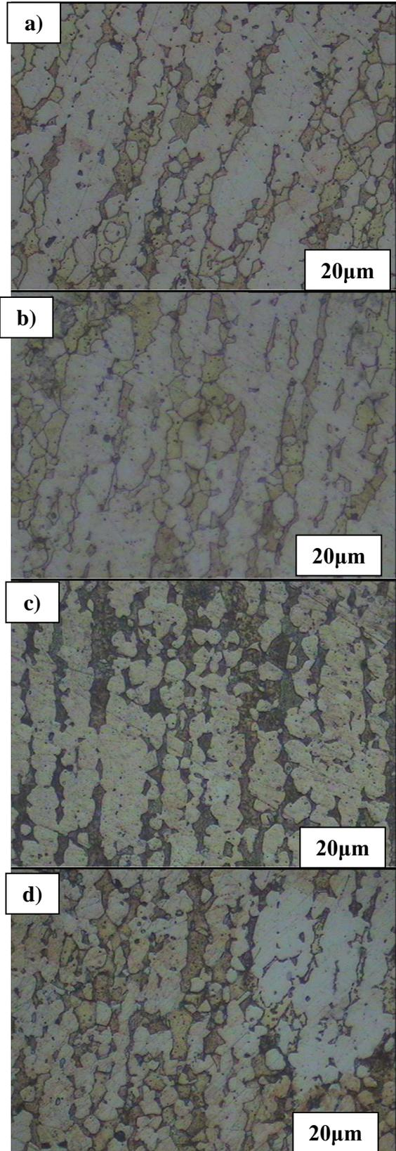
**Fig. 4.1** the microstructure of alloy at various pulsed times for 200°C
