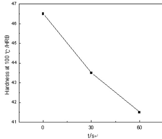
Fig.3.2 micro hardness curve of alloy at various pulsed time for 100°C
