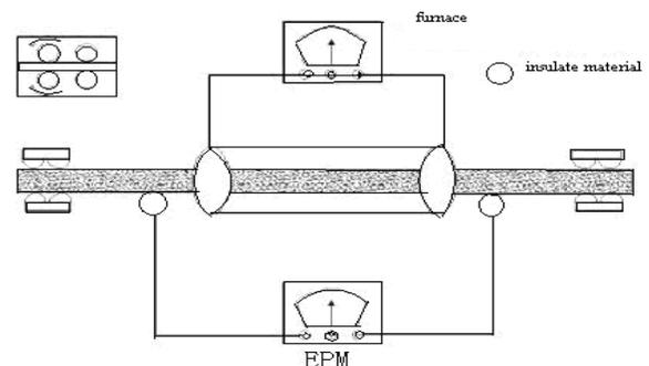
Fig 1 the sketch of annealing process aided by the electric pulse
