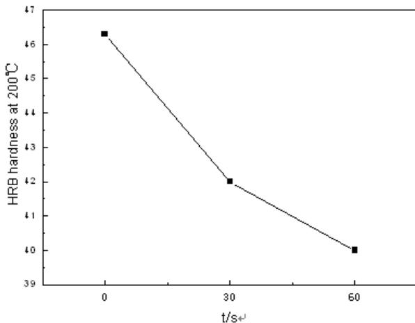
**Fig. 4.2** micro hardness curve of alloy at various pulsed time for 200°C
