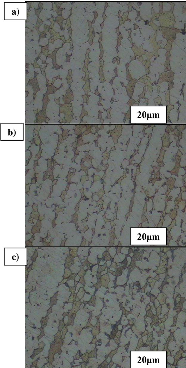
Fig. 3.1 the microstructure of alloy at various pulsed times for 100°C (a) 0s (b) 30s (c) 60s
