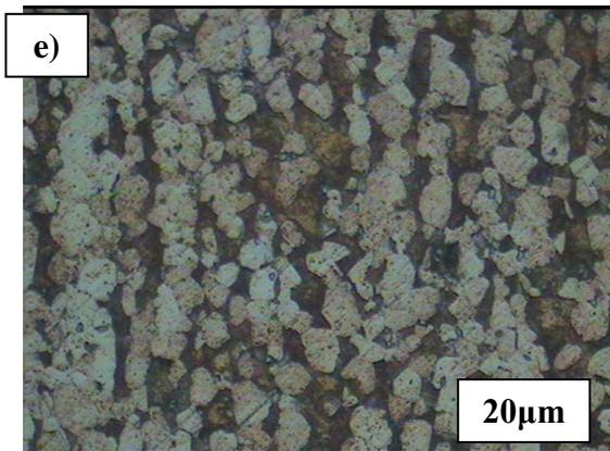
**Fig. 5.1** the microstructure of alloy at various pulsed times for 300°C (a) 0s (b) 30s (c) 60s (d) 90s (e) 120s
