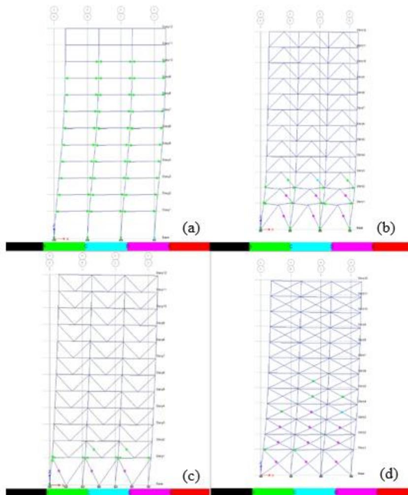
**Figure 6** Plastic hinge formation in 12 storey frame with and without bracings
