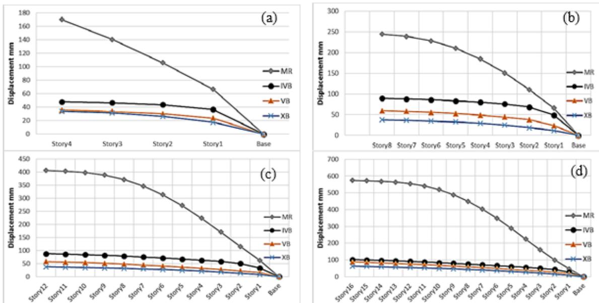
Figure 8 Storey displacement of MR, IVB, VB and XB for (a) 4 (b) 8 (c) 12 (d) 16 Storey
