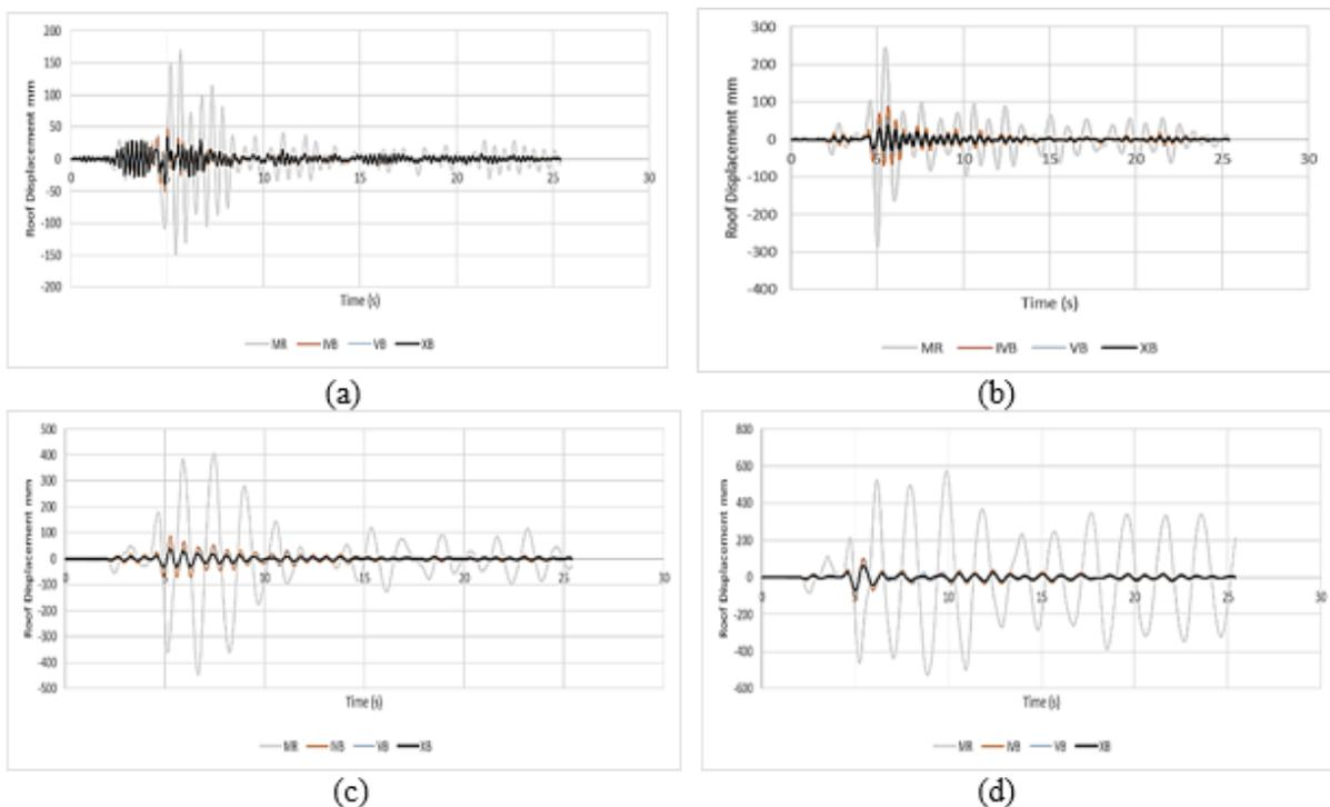
Figure 9 Roof displacement time history response of braced and unbraced frames for (a) 4 storey (b) 8 storey (c) 12 storey (d) 16 storey
