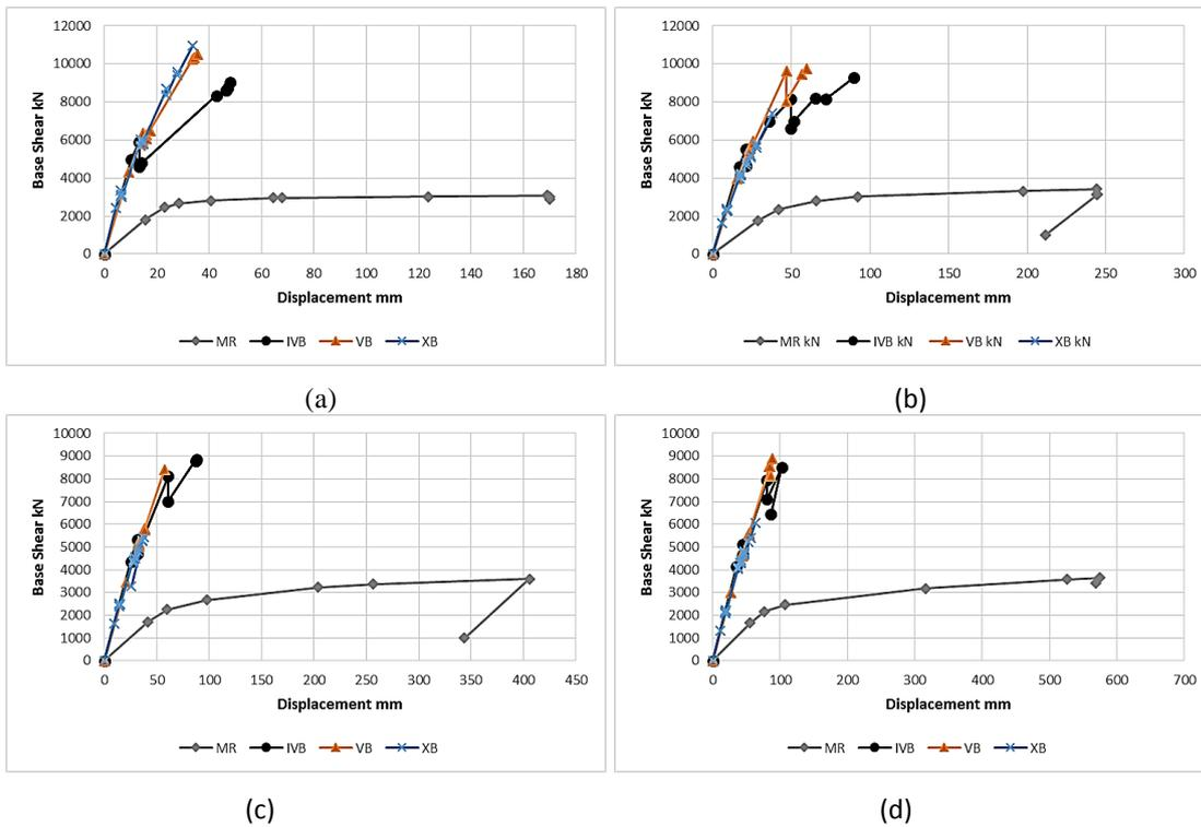
**Figure 2** Capacity curves of braced and unbraced frames for (a) 4 (b) 8 (c) 12 (d) 16 Storey
