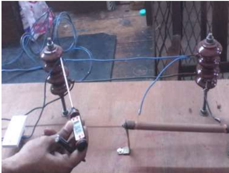
Figure 3. Testing of Temperature on insulator
