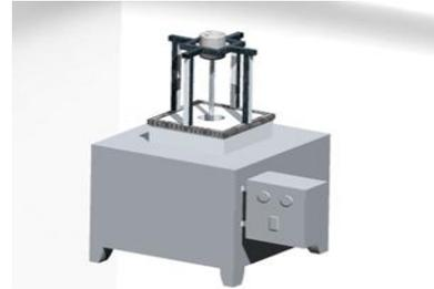
Figure 3 Final experimental setup of stir casting machine designed in CREO
