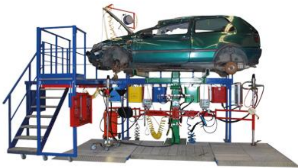
Fig. 1. SEDA Single Station drainage system
