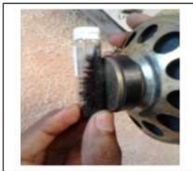
*Figure 4 Manufactured magnetic Iron nano particles*
