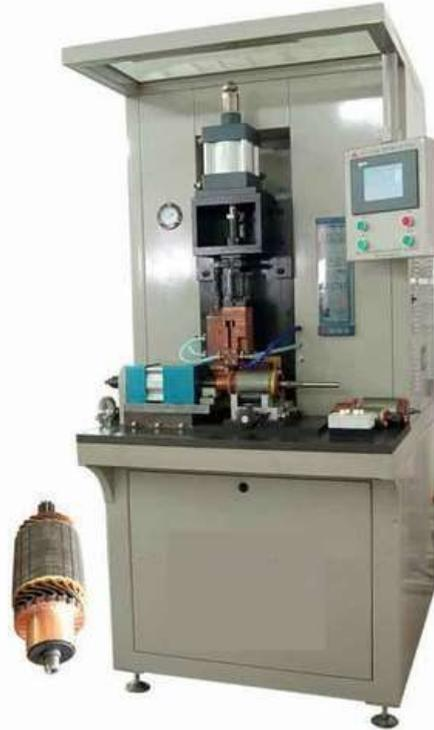
**Figure1: Commutator Fusing Machine**
