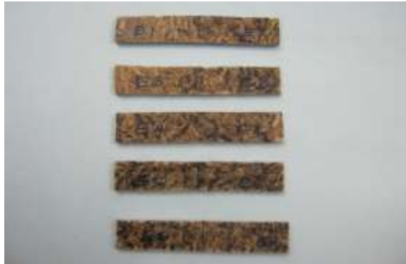
Fig 6.4 Specimen for impact Impact strength=maximum energy absorbed/area of cross section
